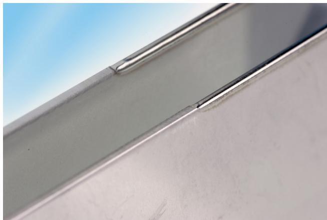
Image 2: Partially laser-rounded sheet edges made of stainless steel (sheet thickness 1.5 mm).
