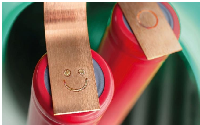
Image 1: One of the topics at LSE'20: efficient laser joining for contacting batteries. © Fraunhofer ILT, Aachen, Germany.
