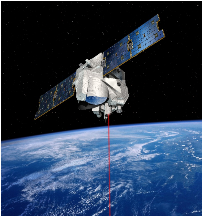
Picture 1: Representation of the MERLIN instrument based on the Myriade satellite platform. © CNES/illustration David DUCROS, 2016.
