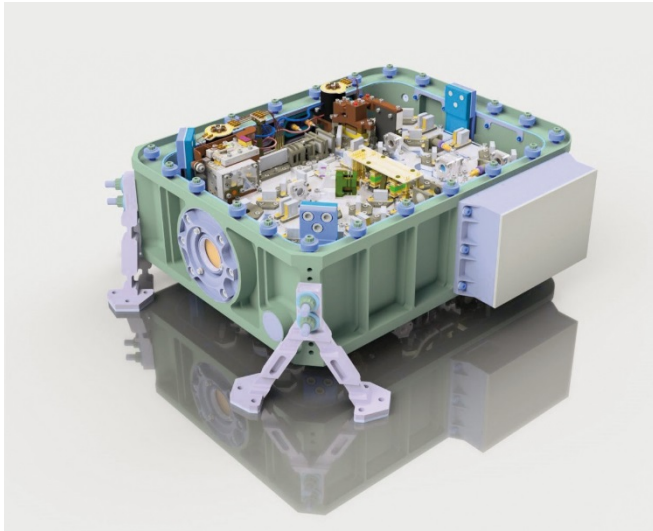
Picture 2: The LIDAR system for the MERLIN mission incorporates all components from the pump laser to the frequency conversion in a particularly compact design suitable for space operation. © Fraunhofer ILT, Aachen, Germany.
