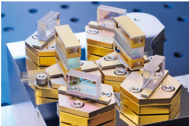
Picture 3: Designed using new soldering techniques: an optical parametric oscillator (OPO) for the MERLIN-LIDAR system. © Fraunhofer ILT, Aachen, Germany.
