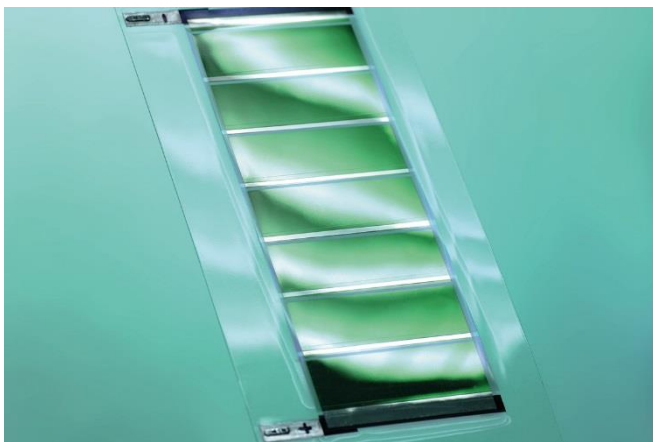
Picture 2: Flexible and organic: A semifinished flexible solar cell is produced on a roll-to-roll system using laser structuring, and will then be finished in a printing process. © Fraunhofer ILT, Aachen, Germany.
