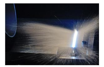
Image 1: Structuring a metal probe with a high-power fiber laser in preparation for a metal-plastic bond. © Fraunhofer ILT, Aachen, Germany.
