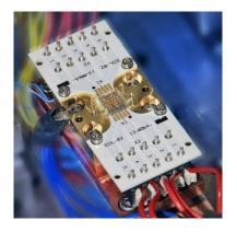
Picture 2: Mounting of individually addressable diode lasers with rear and front facet access for CBC.
