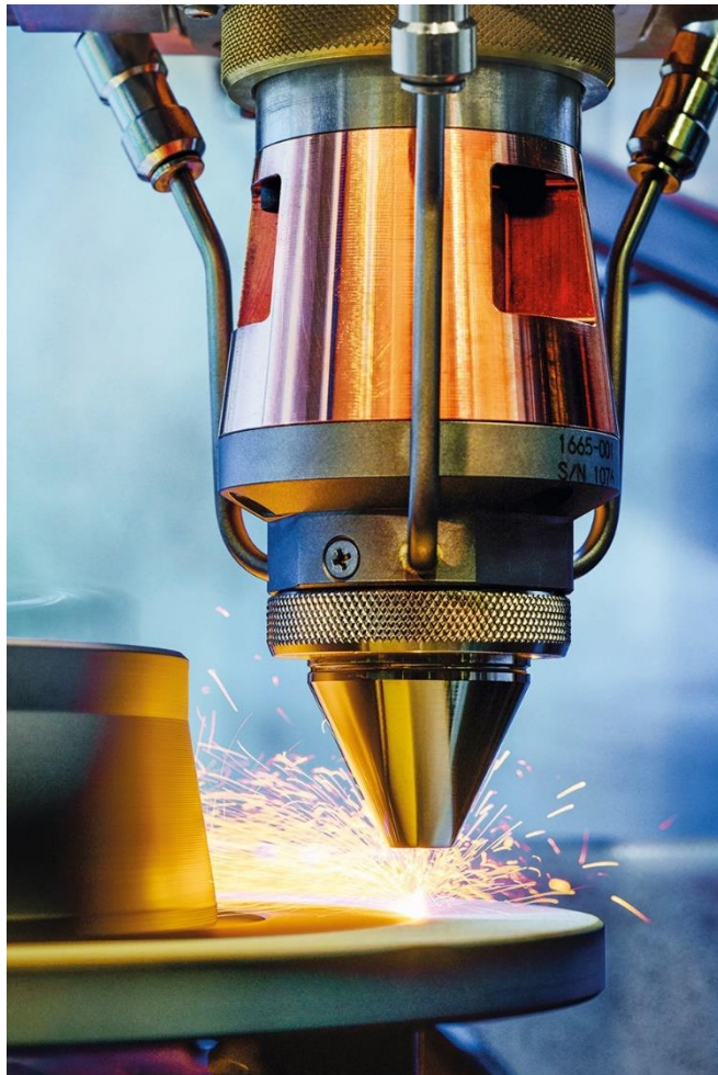
Image 3: The LMD technology process principle can be transferred to almost any system kinematics. It can be used to apply extremely hard coatings that are particularly stable over the long term. © Fraunhofer ILT, Aachen, Germany / Volker Lannert.
