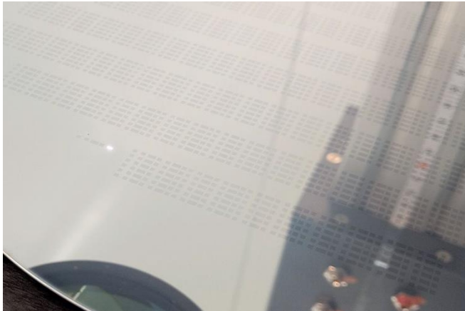
Image 3: Process image of the selective laser crystallization process for silicon wafers developed by Fraunhofer ILT. © Fraunhofer ILT, Aachen, Germany.
