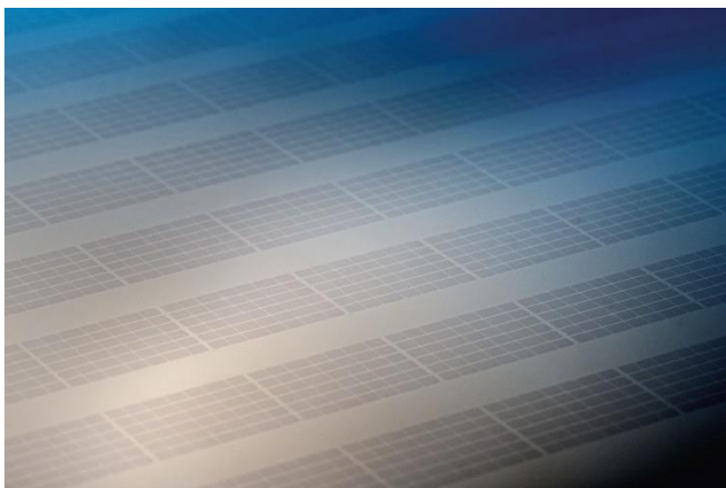
Image 2: Detailed view of the silicon arrays selectively laser-crystallized by Fraunhofer ILT. © Fraunhofer ILT, Aachen, Germany.
