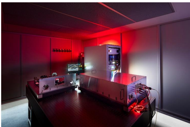
Image 1: With QuTech, Fraunhofer ILT is developing e.g. key components for the quantum internet (shown here: laboratory prototype for a low-noise quantum frequency converter). © Fraunhofer ILT, Aachen, Germany.
