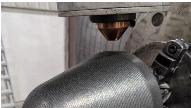
Image 2: Wear parts like this stone crusher tooth with an outer diameter of about 140 mm are restored with the LMD process. Thanks to AI, the processes for repairing irregular surfaces shall be optimized. © Apollo Machine and Welding Ltd, Canada.
